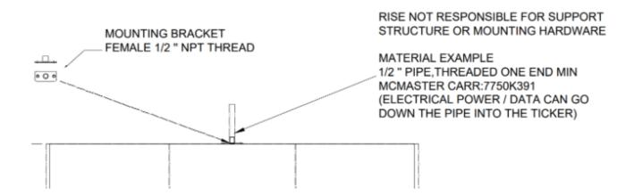
1. Loosely thread the  $\frac{1}{2}$ " NPT female adapter (shown below) onto the  $\frac{1}{2}$ " NPT support (male), do not fully tighten. NPT support not included.
