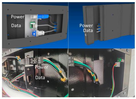
7. The pre-loaded message should start at section A1 and scroll continuously across the entire sign from right to left. If the message doesn't properly scroll through all sections check the data and power cable connections between sections (steps 3 and 4 above).
